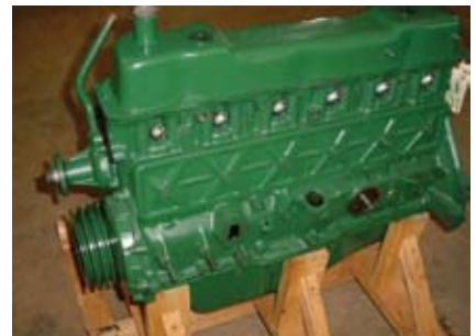
Different than most replacement engines, this HEC model to replace Ford F300, ships with complete sheet metal, including a center-sump oil pan, a high flow water pump and a v-belt front dampner.
