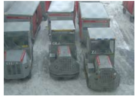
The HEC 4.9 liter can be installed on airport vehicles because it's the identical engine, with the same form-factor and bolt pattern as the original.
